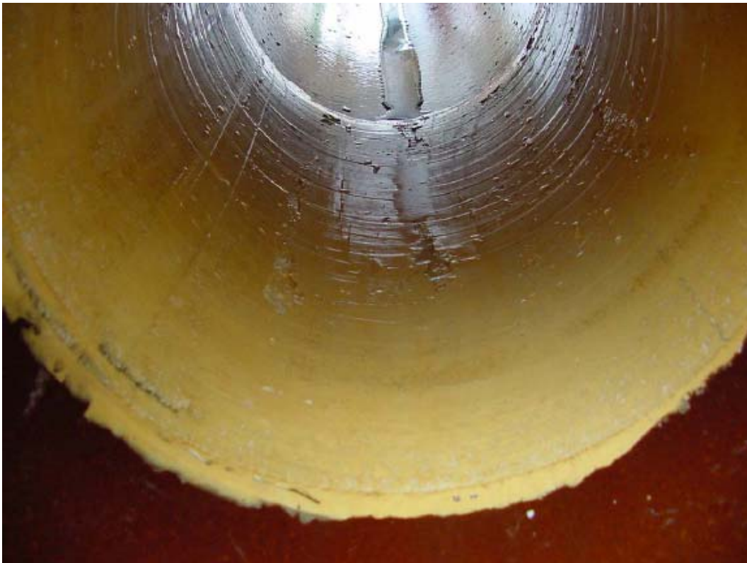
Picture 8: epros patch liner H1263-2.1 after completion of 30 jetter cycles at 80 bar
