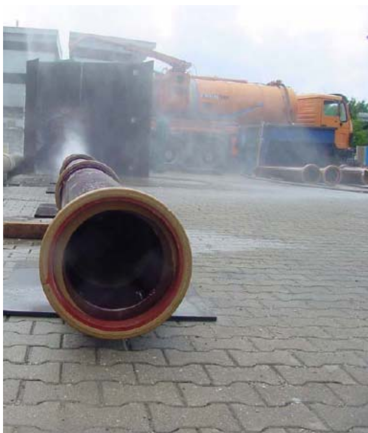
Picture 1: Set-up for the Hamburg Model Jetter Test
