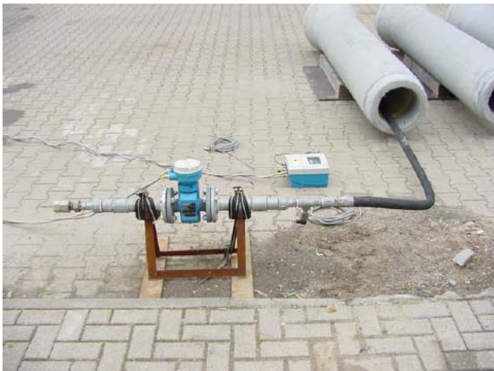
Picture 4: Magnetic inductive flow meter for monitoring the flow rate during testing
