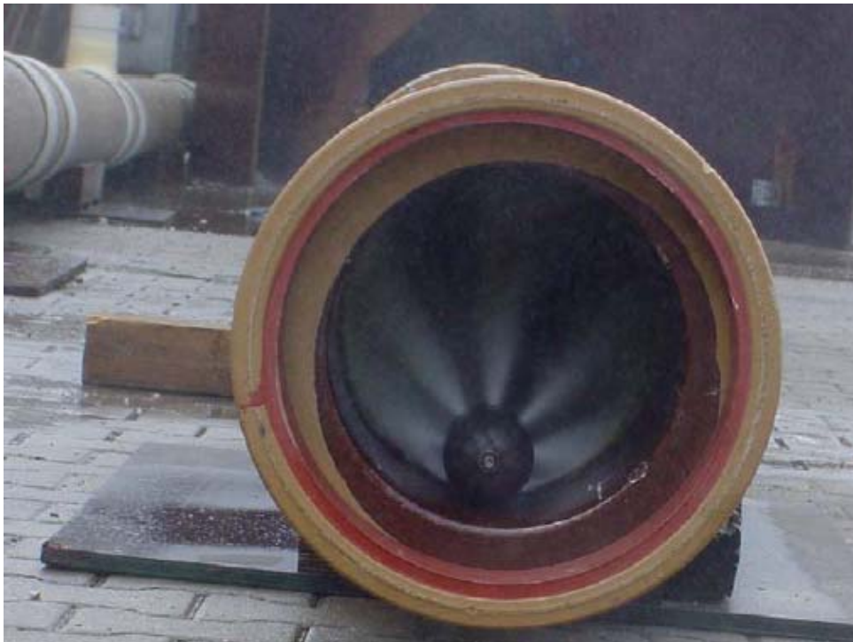
Picture 2: Punctual stationary load by jetter stop (for 3 minutes)
