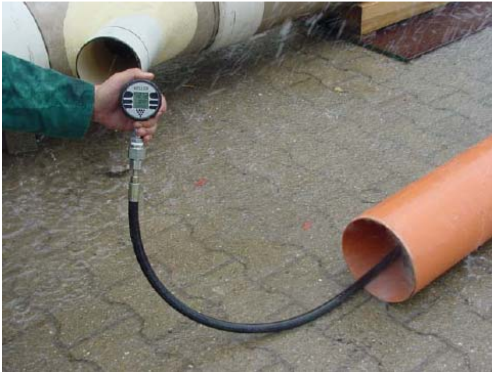
Picture 3: Pressure sensor for checking the water pressure at the nozzle
